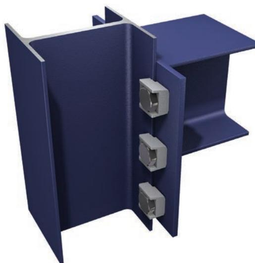
Connecting a horizontal beam with a perforated end plate to the vertical beam
