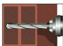
3. Holes to be drilled perpendicular to the surface of the base material by using a hard-metal tipped hammer drill bit. Drill a hole, with drill method according to Annex C4 – C39, into the base material, with nominal drill hole diameter and drill hole depth acc. to the size and embedment depth required by the selected anchor. In case of aborted drill hole the drill hole shall be filled with mortar.
