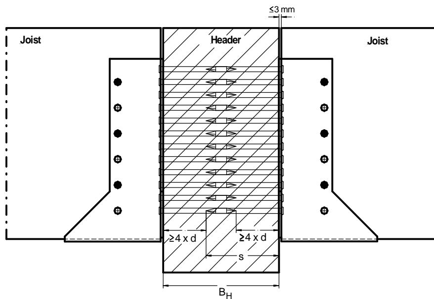
**Joist hanger connected to concrete, lightweight concrete
