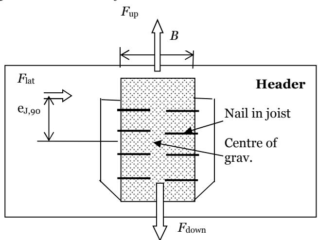
It is assumed that the header beam is prevented from rotating. Similarly it is assumed that the concrete structure or the steel member to which the joist hanger is bolted does not rotate. If the header beam only has installed a joist hanger on one side the eccentricity moment  $M_v = F_d \cdot (B_H / 2 + e_{J,0})$  shall be considered. The same applies when the header has joist hanger connections on both sides, but with vertical forces which differ more than 20%.
