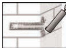
**4.** Blow out from the bottom of the bore hole two times. Attach the brush to a drilling machine or a battery screwdriver, brush the hole clean two times, and finally blow out the hole again two times.
