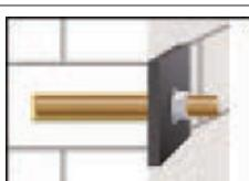
**9.** After full curing, the fixture can be installed with up to the max. installation torque (see parameters of brick Annex C4 to Annex C45) by using a calibrated torque wrench.
